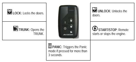
N.B.: Pressing TRUNK and LOCK buttons simultaneously will activate the AUX 1 output. Pressing TRUNK and UNLOCK buttons simultaneously will activate the AUX 2 output.
