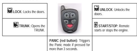
N.B.: Pressing TRUNK and LOCK buttons simultaneously will activate the AUX 1 output. Pressing TRUNK and UNLOCK buttons simultaneously will activate the AUX 2 output.
