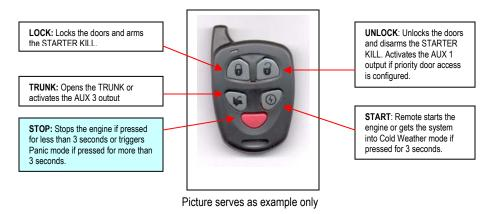
N.B.: Pressing the LOCK and UNLOCK buttons simultaneously will activate the AUX 2 output.
