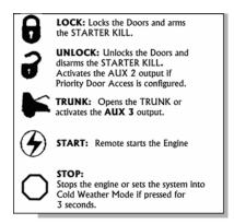
Note: Pressing the LOCK and UNLOCK buttons at the same time will activate the AUX2 output.
