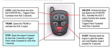
**Note:** Pressing the LOCK and UNLOCK buttons at the same time will activate the AUX 2 output. Remote-starting Your Vehicle
