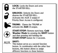
**Note:** Pressing the **SHIFT** and **LOCK** buttons at the same time will activate the **AUX 2** output.
